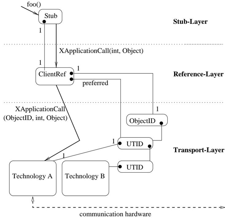
**Fig. 3.** The three layers of the KaRMI design are shown. A method call is handed from the stub to its reference object (`ClientRef`). The reference object has an `ObjectID` which in turn points to a chain of `UTIDs`. Each `UTID` (unique technology identified) has a pointer to the corresponding technology object that talks to the underlying communication network.
