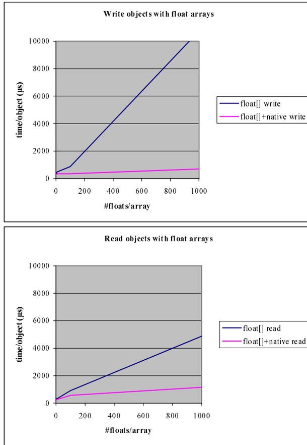
Fig. 2. Serialization of float arrays (same benchmark setup).
